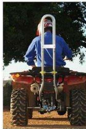
Crush protection devices can be fitted to a quad bike to provide a survivable space should a rider be pinned underneath it. Data reveals that, in many of the work-related quad bike accidents each year, the worker is crushed or unable to escape due to the weight of the bike, contributing to fatal or life-changing injuries. A CPD provides some protection in the event of a quad bike roll-over.
